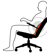
STANDARD SUPPORT - RECLINED As you recline in a standard office chair, the backrest pulls away from you, creating a gap in lumbar support.
